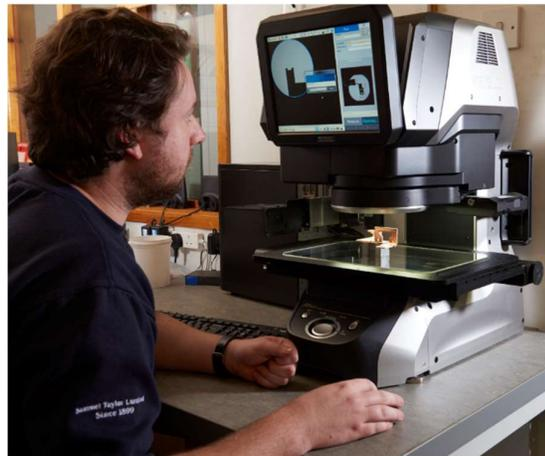
“The Keyence machine came in addition to our CMM, which is also a great piece of kit. Put simply, it eliminates human error. The challenge is to make sure it is well programmed, and it understands what it is supposed to look for, which is our job to ensure happens” adds Bogdan.
