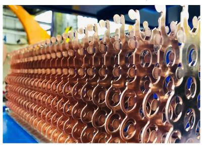
"We made certain adjustments within the stamping process to increase the accuracy of busbar production. For example, we established a customised press line to produce busbars with the ability to switch modules on and off, enabling us to deliver optimised pressure but spread over a row of two or three cells - a pattern that repeats row by row through the part.
